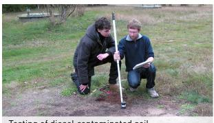
Testing of diesel contaminated soil
