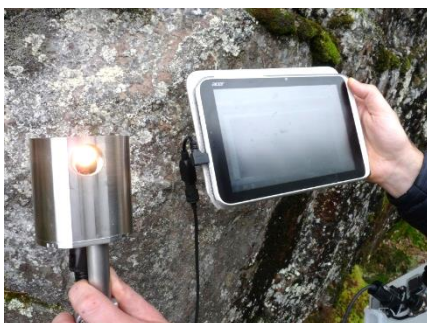
Fig. 1: REO-Explorer, composed of spectrometer unit, measurement head, optical fibres and tablet PC
