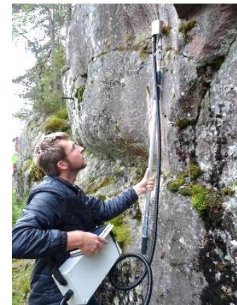
Fig. 2: Field measurements with prototype of REO-Explorer
